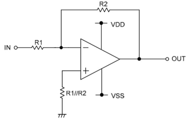
Figure 12. Inverting amplifier circuit
