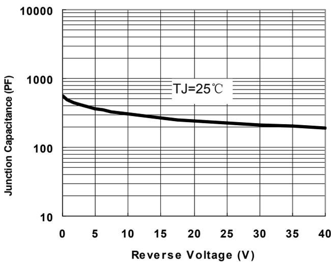
**Fig.1-Typical Junction Capacitance**
