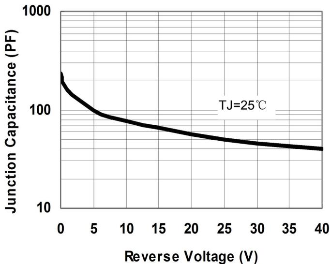
Fig.1-Typical Junction Capacitance
