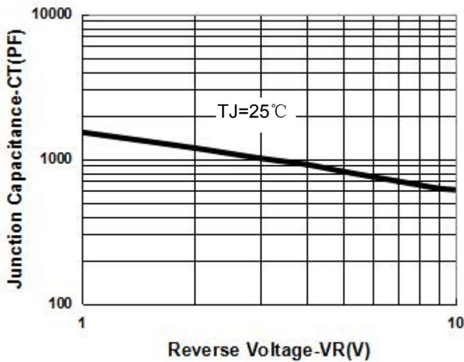
Fig.1-Typical Junction Capacitance
