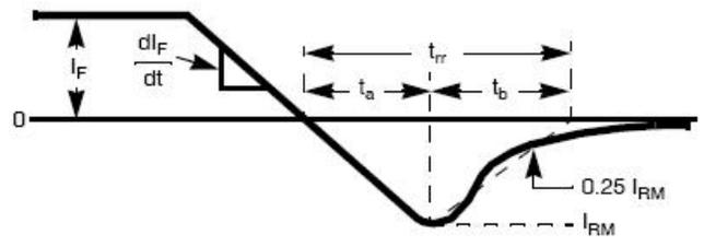
**Figure 11. Diode Reverse Recovery Waveform**
